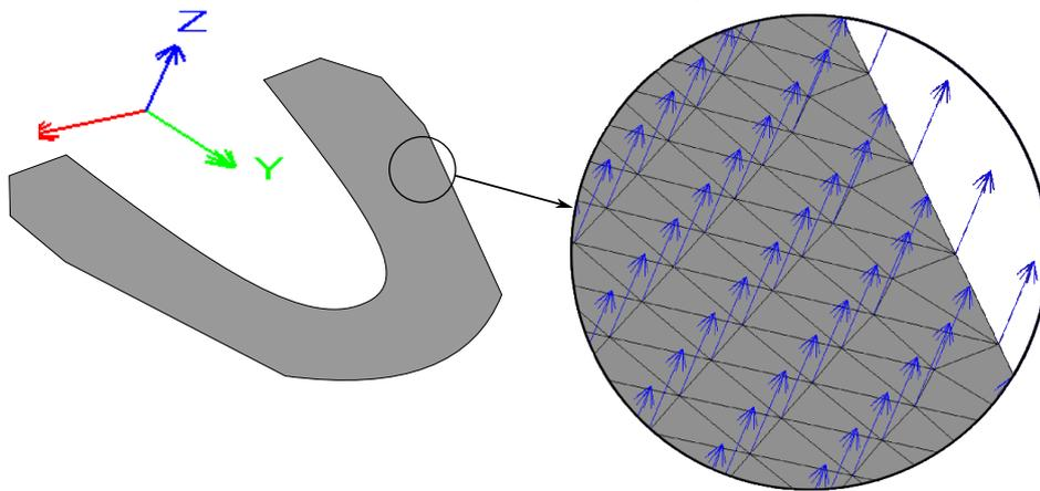
Figure 2.4: Detail of a mesh (direction of normals)
