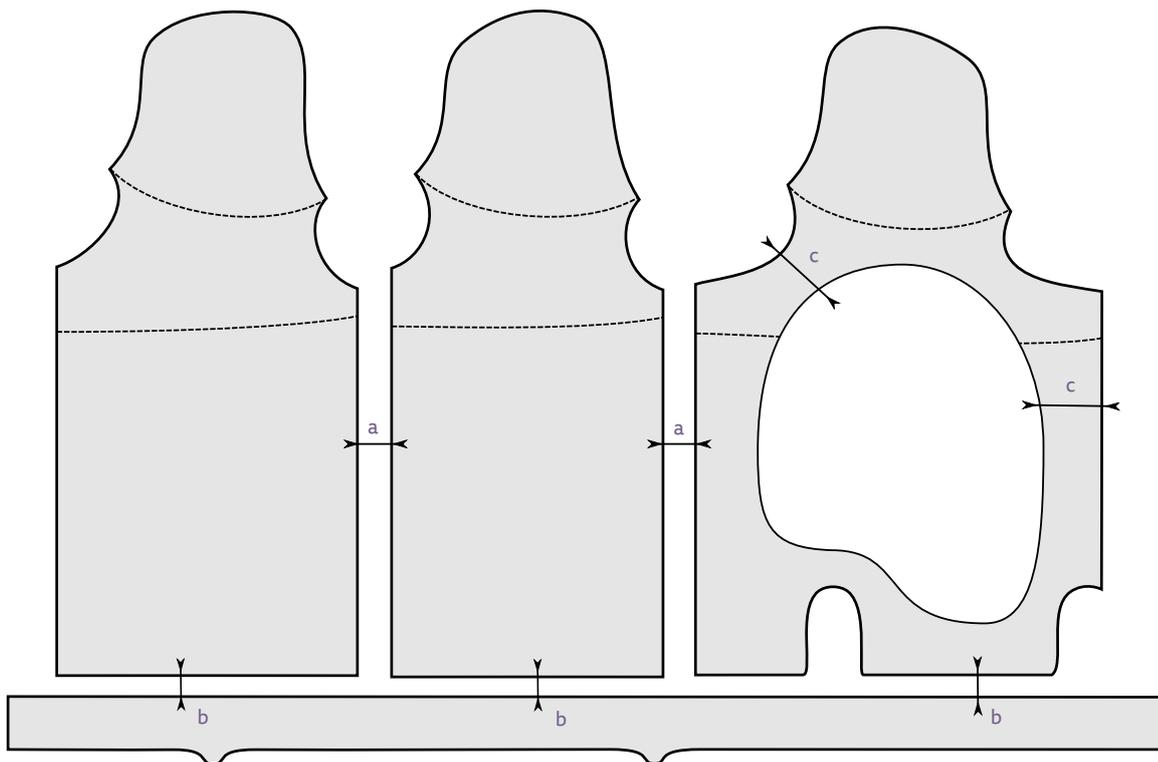
Figure 2.6: Construction parameters for plate-type models
