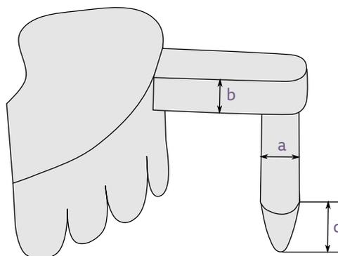
Figure 3.1: Construction parameters for support pins
