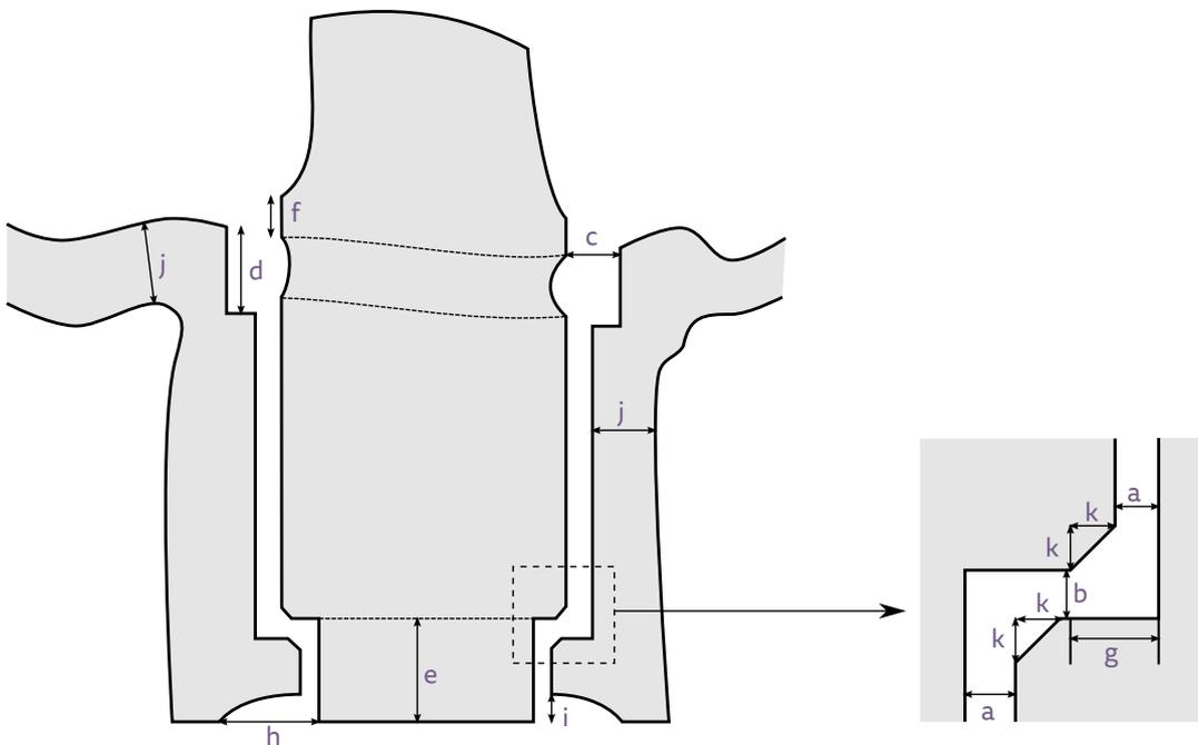
Figure 2.7: Construction parameters for plateless models
