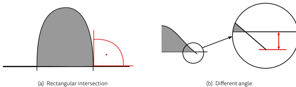
Figure 2.3: Pins intersecting the base plate
