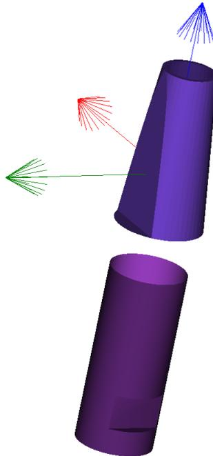
Figure 4.1: Retention mesh and scan abutment in the same coordinate system
