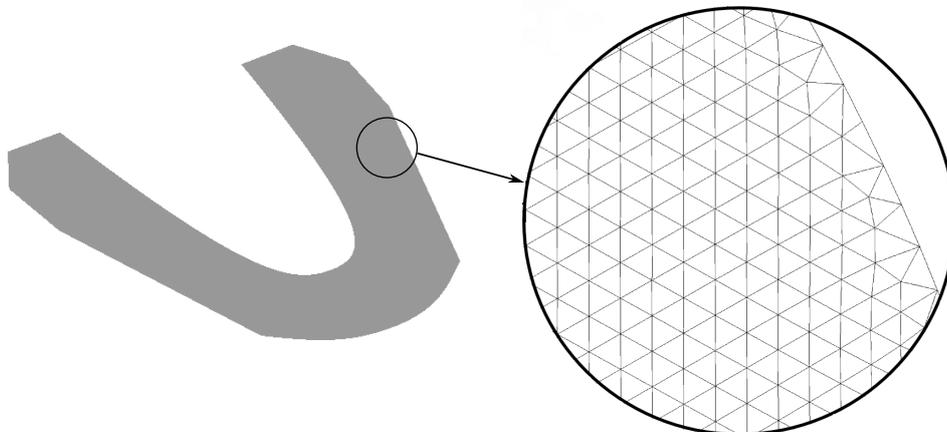
Figure 2.5: Detail of a mesh (triangulation)
