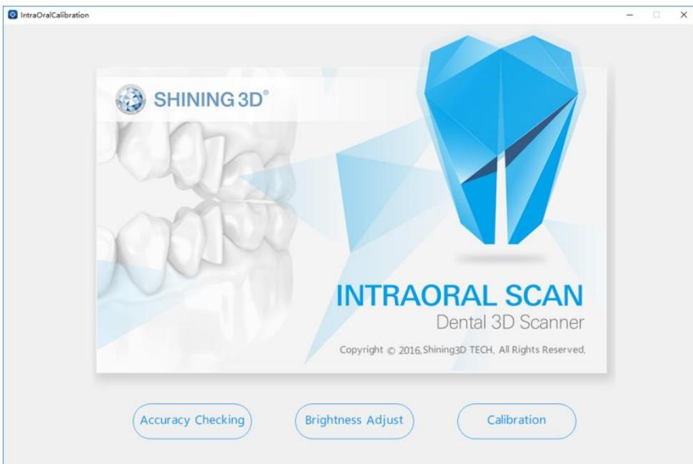
(10) Click Calibration. If the Calibrator was not closely plugged onto the scanner, a warning message would be popped up. So, make sure the scanner be plugged into the calibration firmly before next operation.
