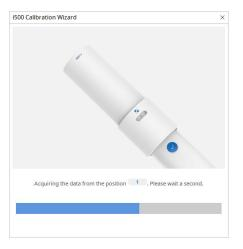
When data acquisition is completed at the position \_\_\_\_, turn the dial to the next position.
