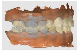
The system will calculate the occlusion alignment based on marked points pairing.
