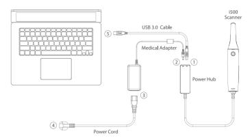
> ① Connect the USB 3.0 Cable to the Power Hub
