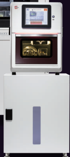
4 axis Wet Custom abutment milling DS200-4WA
